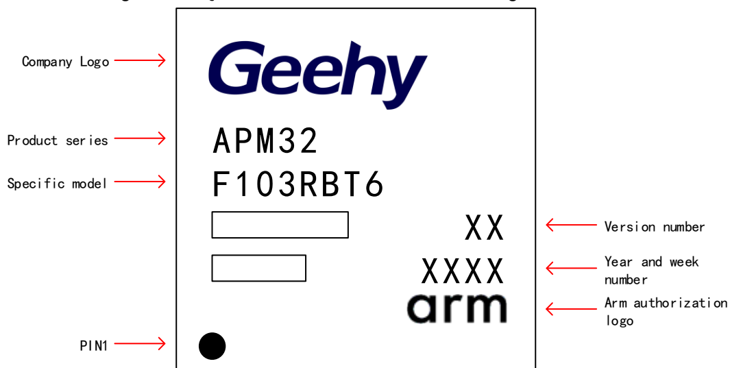
Figure 25 LQFP64 - 64 Pins, 10 x 10mm Package Identification
