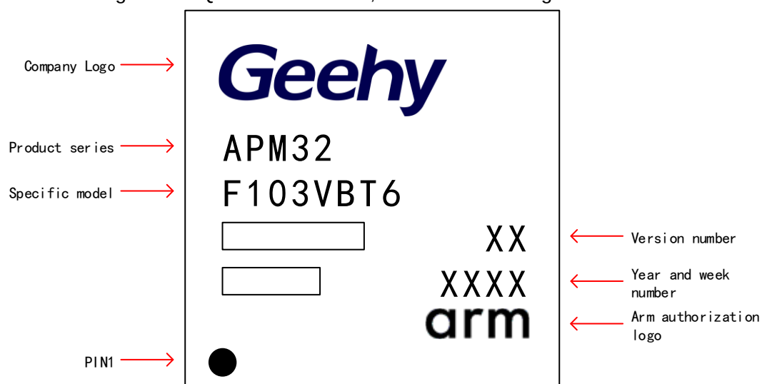
Figure 22 LQFP100 - 100 Pins, 14 x 14mm Package Identification
